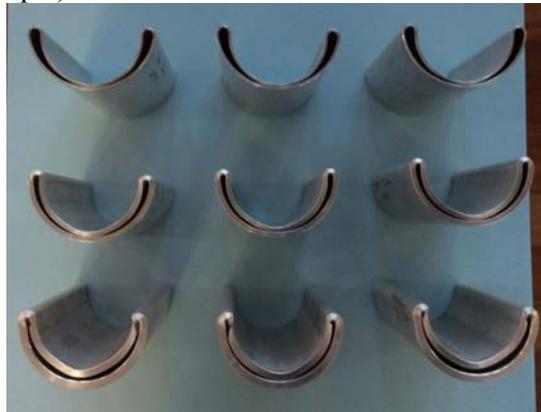
Figure 12. Test Samples ( $D/t$ : 16.2, 23.8 and 47.6) after the CRST
