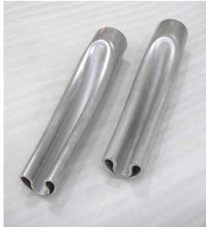
Figure 2. Confined Buckle Propagation with the U-mode Shape of Deformation
