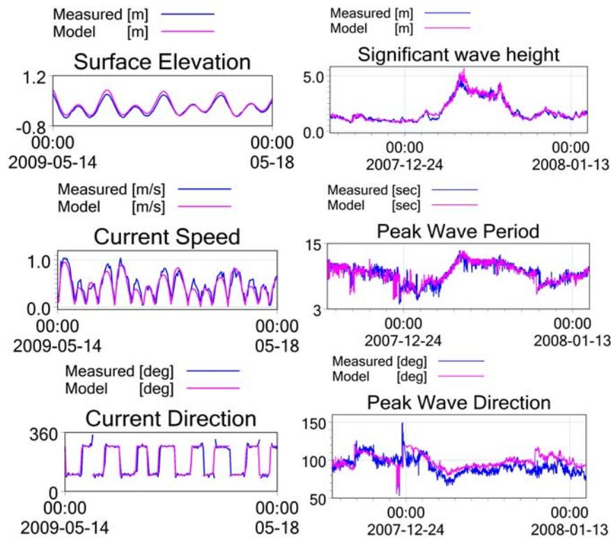
Figure 7. Comparison of hydrodynamics model results and measurements
