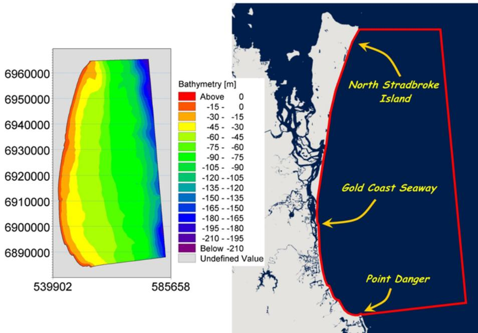
Figure 4. Regional Wave model domain and Bathymetry
