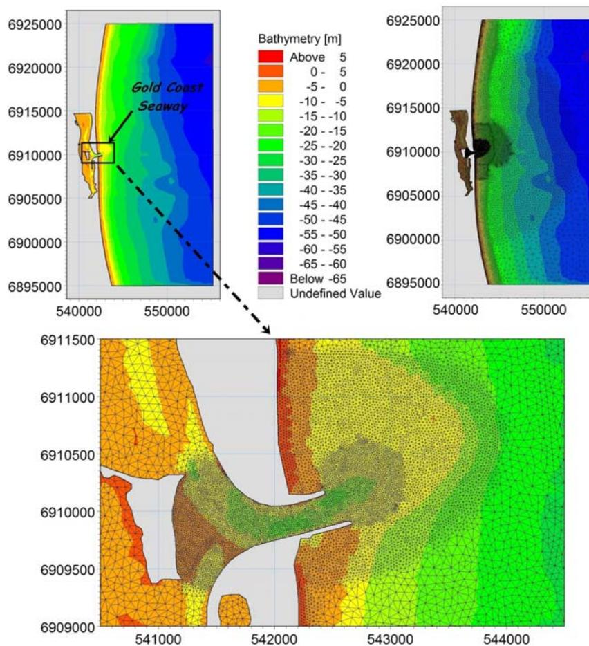
Figure 5. Local HD Model Domain and mesh
