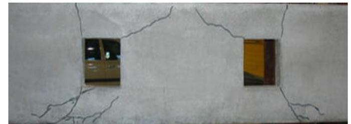
(e) Single point loading case of PC beam with web openings
