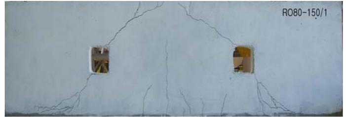
(c) Single point loading case of RC beam with web openings
