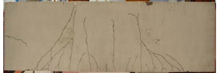
(b) Two points loading case of solid RC beam
