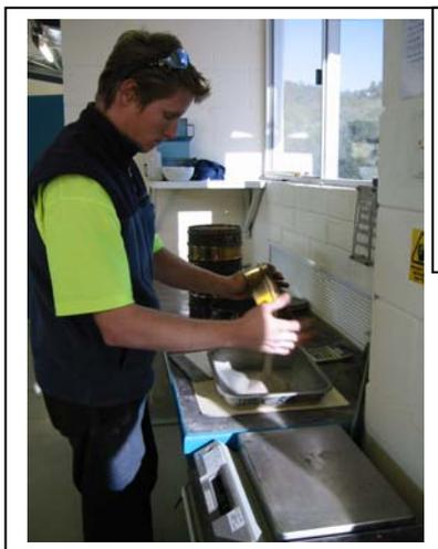
Matt: That's working out one of the gradings, so get the whole weight of the sample and work it back by dividing the total weight by 100 and dividing each separate weight on each sieve by that total weight and then just minusing from 100 down to get the percentage.
