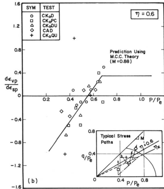
Figure 2.  $(d\varepsilon_{vp} / d\varepsilon_{sp}, p / p_e)$  relationship for a constant stress ratio line from the  $K_0$  consolidation test.
