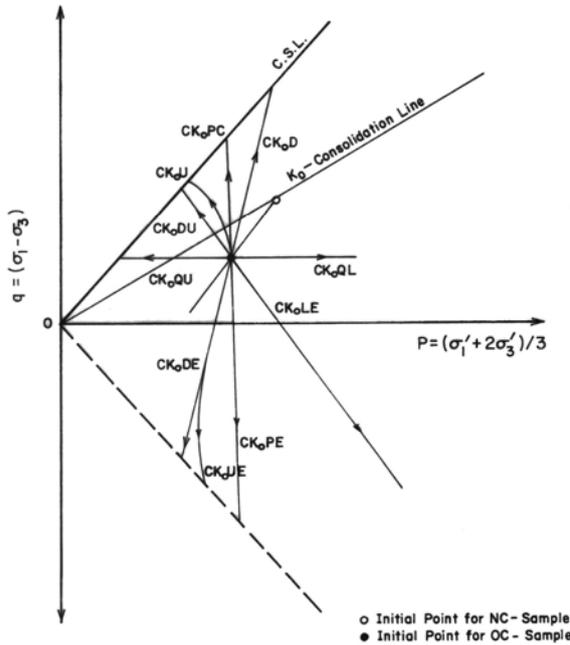
Figure 1. Typical stress path of the behaviour of lightly overconsolidated clay (Kim, 1991)
