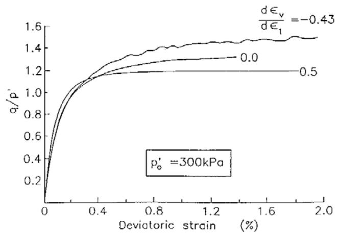
Figure 8. Stress ratio versus strain behaviour of dense sand obtained from constant strain increment ratio paths
