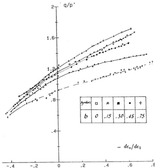
Figure 7. Stress-dilatancy behaviour obtained from constant b tests
