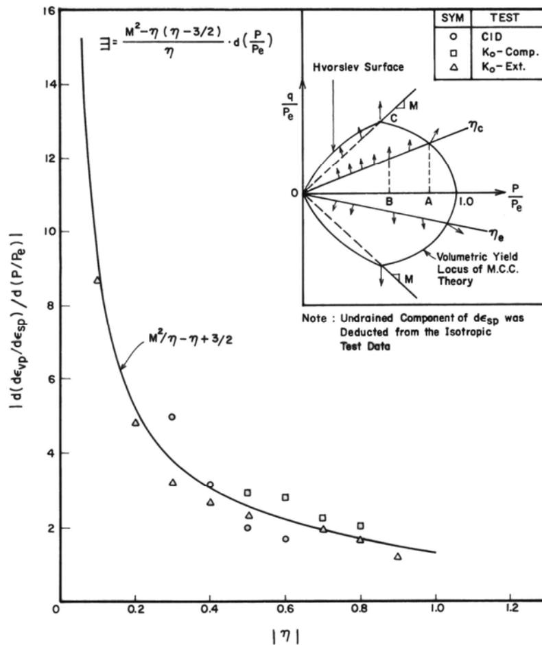
Figure 3. Variation of the  $(d\varepsilon_{vp} / d\varepsilon_{sp}, p / p_e)$  plot with the stress ratio within the state boundary surface.
