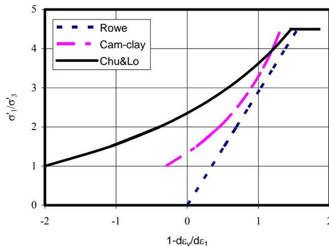
Figure 9. Comparison of different stress-dilatancy relationships
