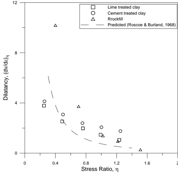
Figure 6. Variation of dilatancy with stress ratio
