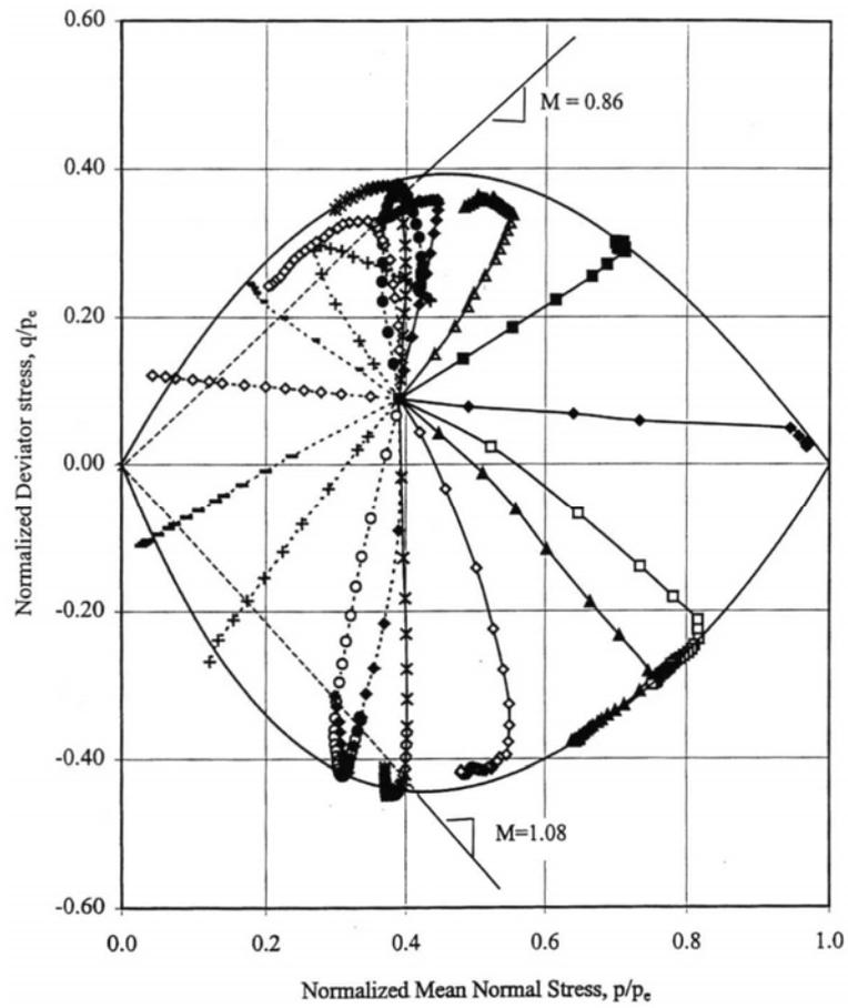
Figure 4. Stress probe paths in  $(q/p_e, p/p_e)$  plot (after Khan, 1999).
