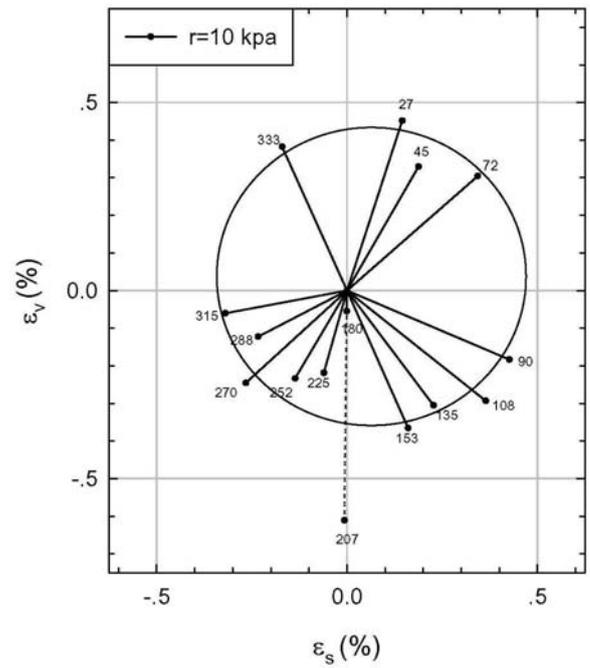
Figure 5b.  $(\epsilon_v, \epsilon_s)$  plot for  $\sqrt{\Delta p^2 + \Delta q^2} = 10$  kpa with fitting (after Pornpong, 2001).
