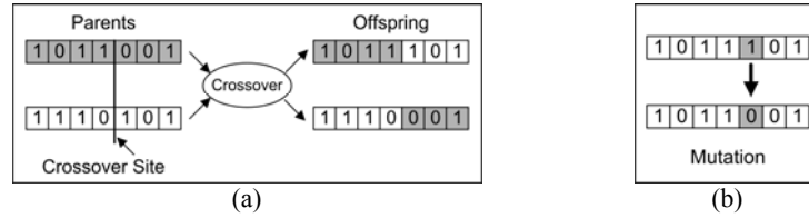
Fig. 5. An example showing (a) 1-point crossover, (b) mutation by 1 bit flipping.
