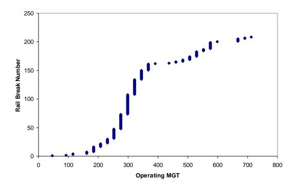
Figure 2: Cumulated Rail break vs accumulated MGT.
