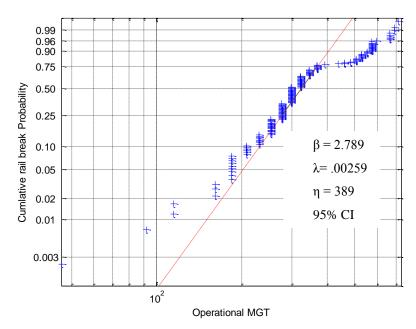
Figure 3: Analysis rail failure data
