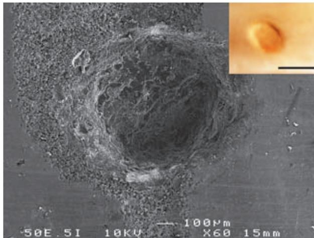
**Fig 1** Crater from 500 mJ laser pulses on the internal dentine surface at 0.5 ml/min water flow rate show no charring, fissures, or microfractures of the surrounding dentine. The margins of the crater are perpendicular (SEM 60X magnification; inset: light micrograph with scale bar = 1 mm).
