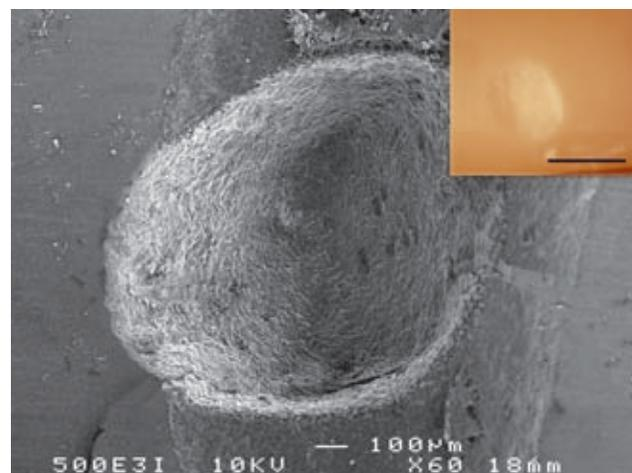
**Fig 4** Crater from 500 mJ laser pulses on the external dentine surface at 1.5 ml/min water flow rate also show no charring, but margins of the crater are bevelled (SEM 60X magnification; inset: light micrograph with scale bar = 1 mm).
