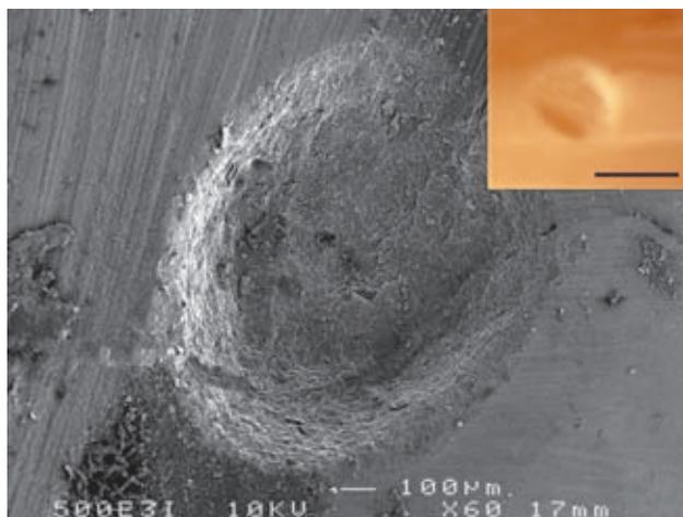
**Fig 3** Crater from 500 mJ laser pulses on the internal dentine surface at 1.5 ml/min water flow rate show no charring, and perpendicular margins (SEM 60X magnification; inset: light micrograph with scale bar = 1 mm).
