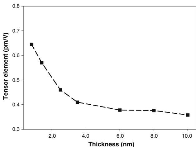
**Fig. 3** Second-order susceptibility as a function of sample thickness for a doped sample
