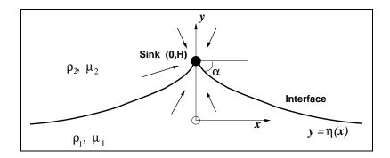
Figure 1. Schematic of the flow into a link sink from two layers of different density - supercritical flow rate.
