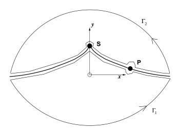
Figure 2. Contours used in formulation of the integral equation. The contours avoid the sink S and the point  $z_0$ , denoted P. The contribution to the integral from the two radial arcs as  $r \to \infty$  is zero, leaving just the integral along the interface.
