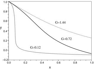
Figure 3. (a) Interface shapes with  $\alpha = -\pi/4$ , for G = 0.12, 0.72 and 1.44 compared with the asymptotic solution given by (22). (b) close-up view of the same showing behaviour near to the sink. Note the steepening of the surface as the nondimensional flow rate, G, decreases.
