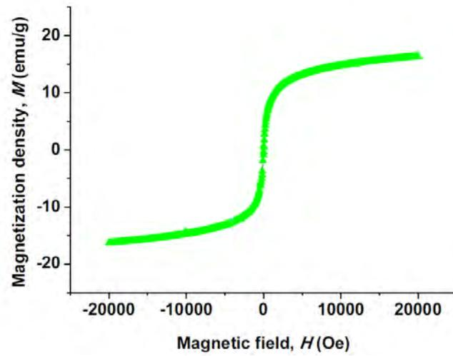
**Fig. S2.** Magnetization curve measured at 300 K for Au@NPF<sub>2</sub>O<sub>3</sub>NC.
