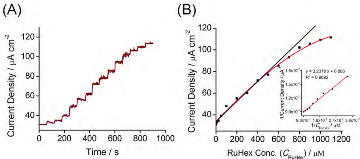
**Fig. S7.** (A) Amperometric responses of GCE/Au@NPFe<sub>2</sub>O<sub>3</sub>NC with the successive addition of RuHex solution (10 to 1100 $\mu\text{M}$ ) into the 0.01M PBS (pH-7); (B) the corresponding calibration plot. Inset of Fig. B: Lineweaver-Burk Model.
