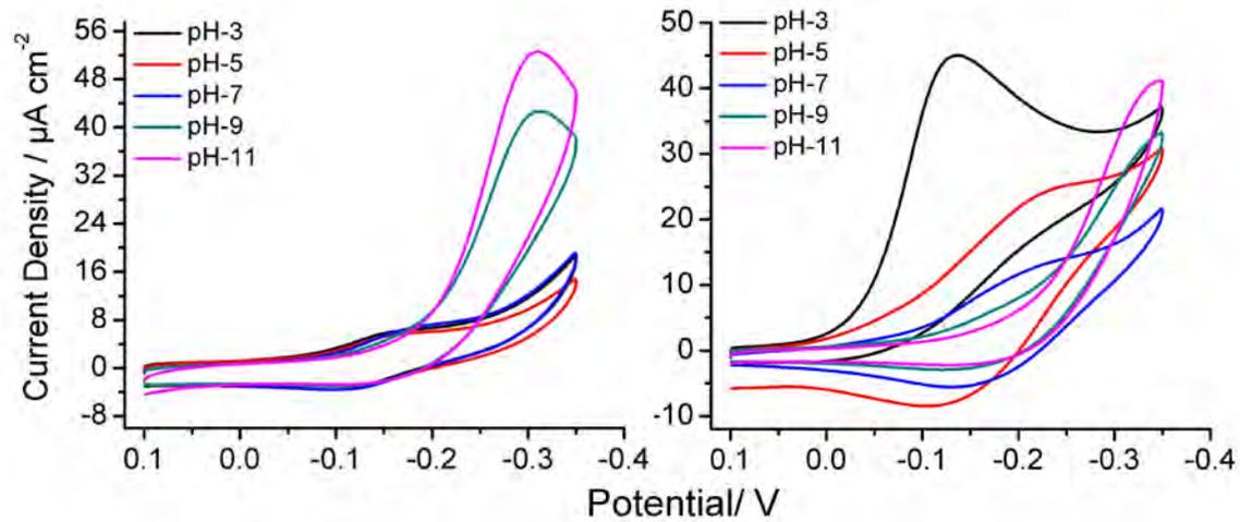
**Fig. S3.** Cyclic voltammograms at GCE/Bare (left) and GCE/Au@NPFe<sub>2</sub>O<sub>3</sub>NC (right) at designated pH from 3 to 11 in the presence of 50 $\mu\text{M}$  RuHex (0.01M PBS, pH-7, scan rate 50mVs<sup>-1</sup>).
