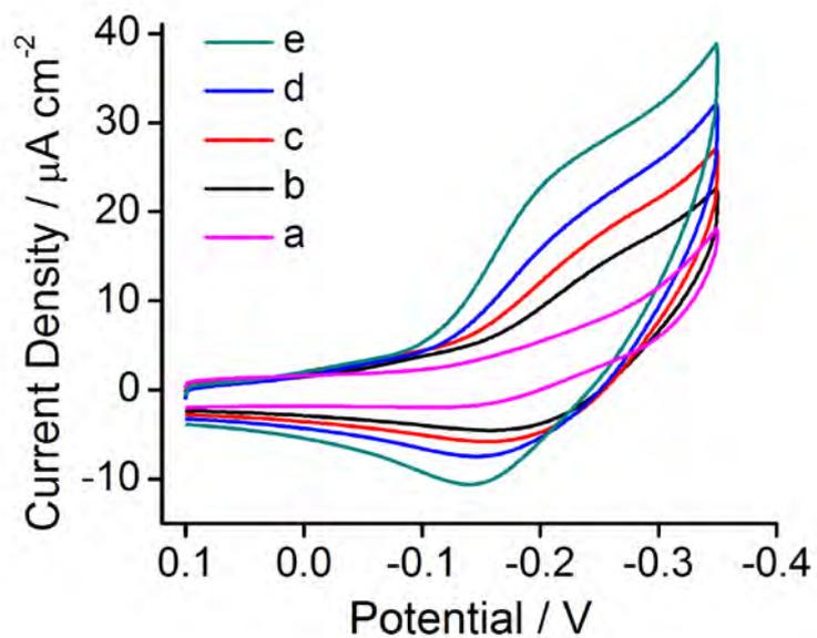
**Fig. S6.** Cyclic voltammograms of GCE/Au@NPF<sub>2</sub>O<sub>3</sub>NC upon successive addition of RuHex (a-0, b-25, c-50, d-100, and e-200  $\mu\text{M}$ ) to the 0.01M PBS (pH-7, scan rate = 50mVs<sup>-1</sup>).
