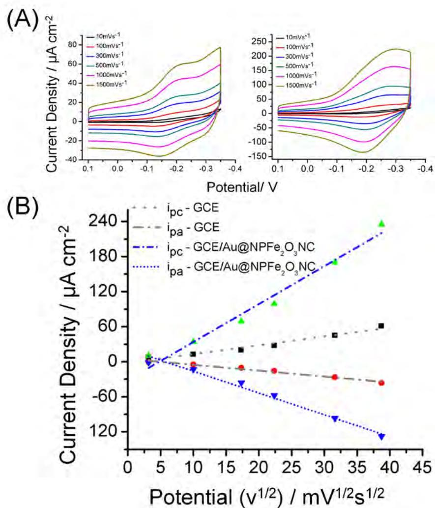
**Fig. S5.** (A) Cyclic voltammograms obtained at GCE/Bare (top, left) and GCE/Au@NPF<sub>2</sub>O<sub>3</sub>NC (top, right) electrodes at different scan rate (50  $\mu\text{M}$  RuHex, 0.01M PBS, pH 7.0). (B) Corresponding curves for  $i_{pc}$  and  $i_{pa}$  (current density) as a function of  $v^{1/2}$ .
