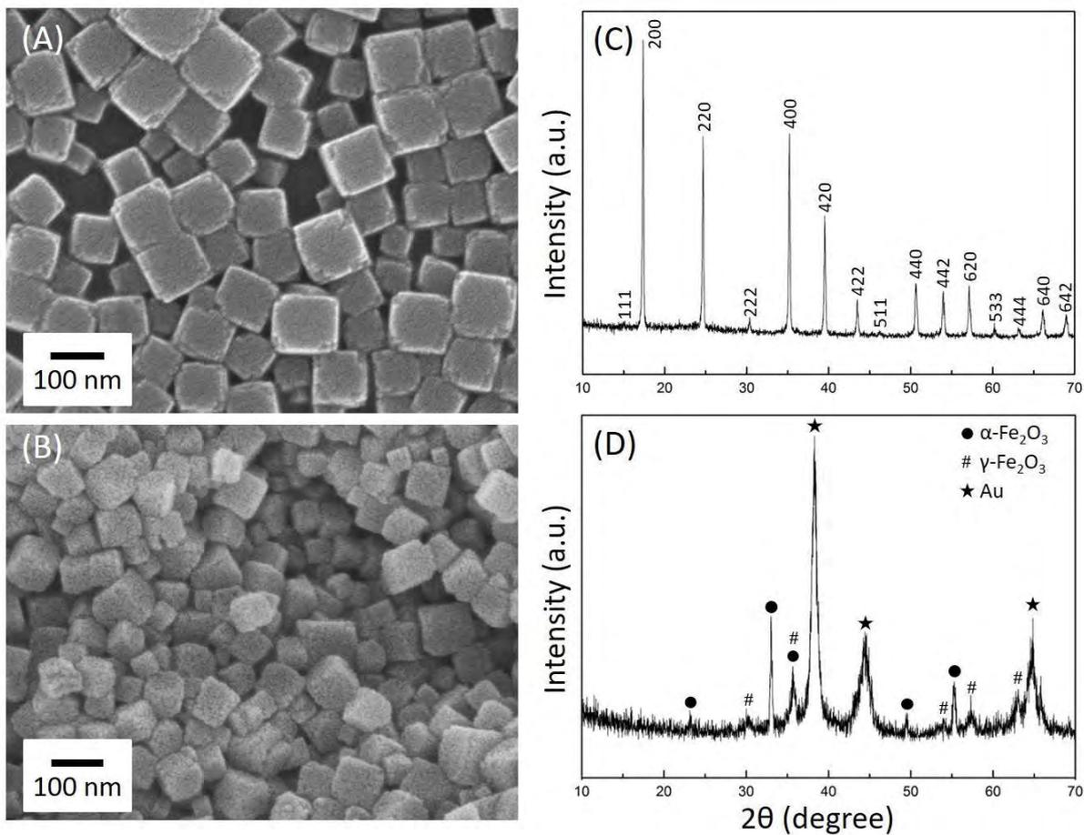
Fig S1. (A-B) SEM images of (A) PB nanocubes and (B) the calcined PB nanocubes. (C-D) Wide-angle XRD patterns of (C) PB nanocubes and (D) Au-loaded nanoporous iron oxide nanocubes.
