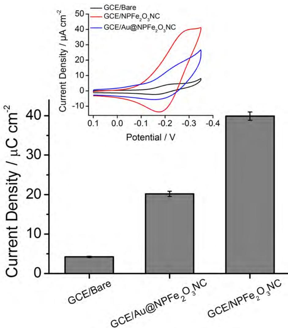
**Fig. S8.** Cathodic peak currents obtained by bare GCE, Au@NPFe<sub>2</sub>O<sub>3</sub>NC-modified-GCE and NPFe<sub>2</sub>O<sub>3</sub>NC-modified GCE at room temperature, in presence of 50 $\mu\text{M}$  RuHex (0.01M PBS, pH-7, scan rate = 50mVs<sup>-1</sup>). Inset, corresponding cyclic voltammogram.
