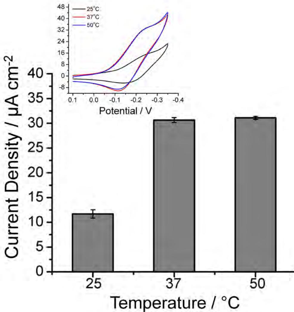
**Fig. S4.** Cathodic peak currents of GCE/Au@NPFe<sub>2</sub>O<sub>3</sub>NC at 25°C, 37°C and 50°C in the presence of 50 $\mu\text{M}$  RuHex (0.01M PBS, pH-7, scan rate = 50mVs<sup>-1</sup>). Inset, corresponding cyclic voltammogram.
