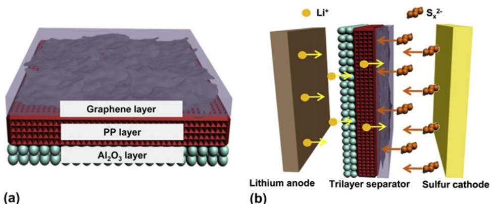
FIG. 3. Schematic illustration of (a) the structure of GPA separator, and (b) Li–S battery with GPA separator. Reproduced with permission from Ref. 106, Copyright 2016, Elsevier.
