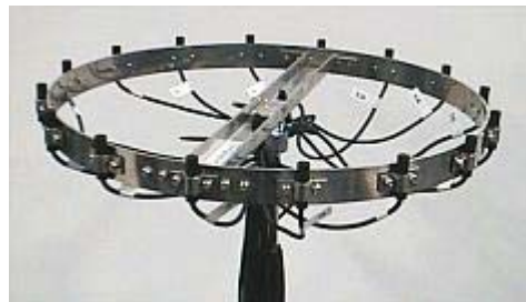
Figure 22 - Circular microphone array with 16 channels [Hiya00]
