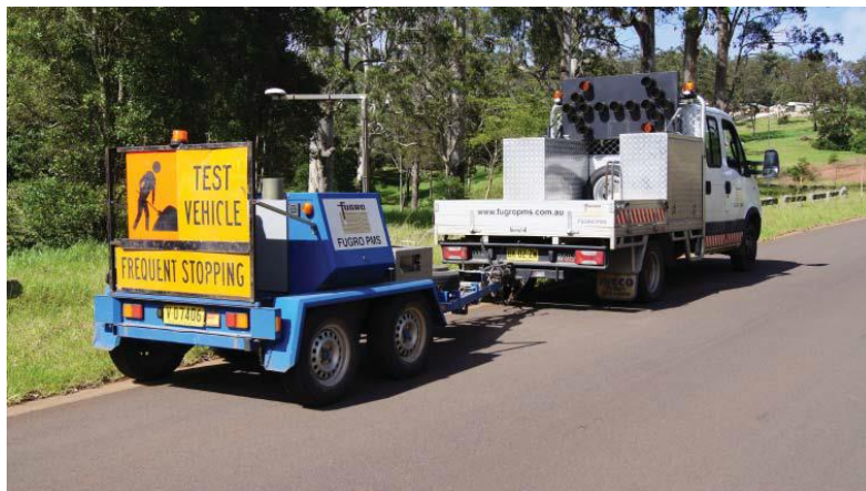
Figure 2.3: Using FWD for pavement strength testing in the outer wheel path (Fugro 2012)
