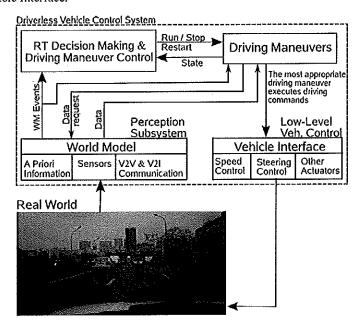
Figure 2. Autonomous vehicle control system.
