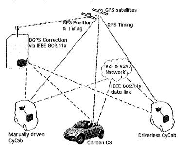
Figure 6. Overview of the example communication setup (adapted from [2]). The autonomous CyCab communicated with a manually driven CyCab and a conventional car.
