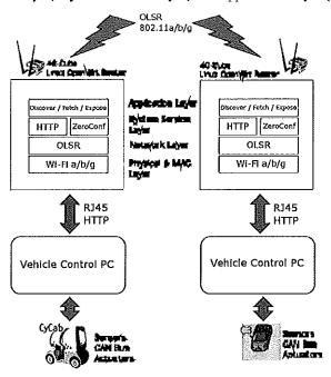
Figure 4. The Cybercars-2 Communication Framework architecture.
