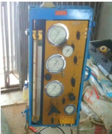
Figure 1 The control unit of the classic Menard pre-bored pressuremeter.
