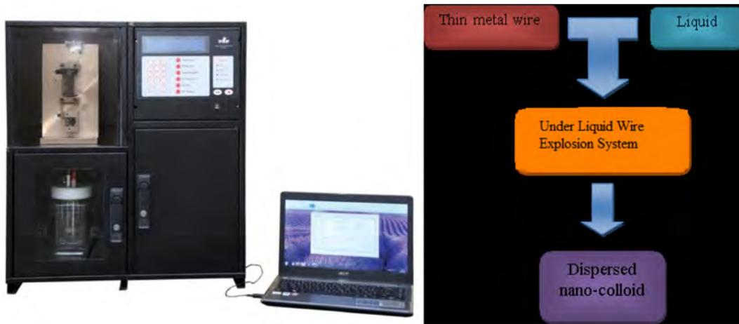
**Figure 1** PNC1K device (left) and a schematic of EEW method (right).
