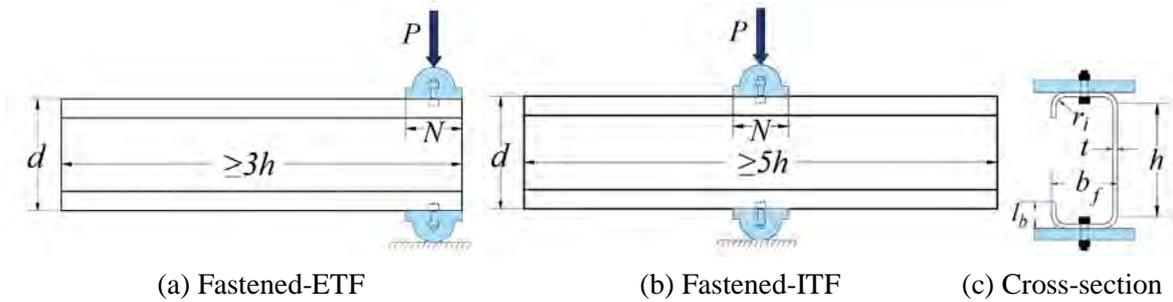
Figure 1: Fastened two flange load cases configuration
