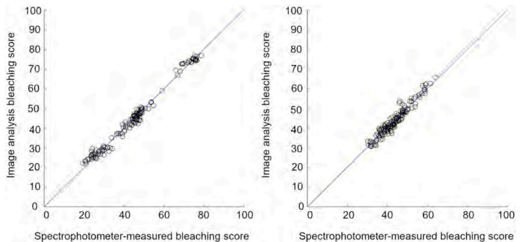
**Fig 4. Performance of image-based bleaching scores.** Bleaching scores assessed by image analysis highly correlated with bleaching scores measured by colour spectrophotometer for (a) the colour sorted samples,  $R^2 = 0.99$ , and (b) the time-course samples,  $R^2 = 0.96$ . Blue lines represent the one-to-one relation.
