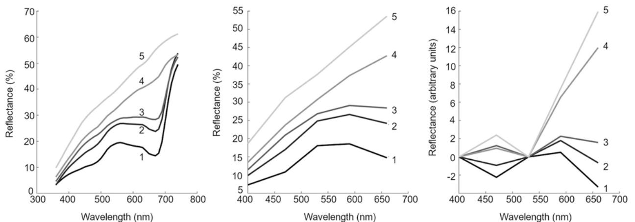
**Fig 1. Spectral response of bleaching.** Example spectra of five green pea genotypes at various stages of bleaching. Dark line (1) represented the least bleached and lightest grey line (5) represented the most bleached. (a) Original spectra measured by spectrophotometer; (b) Spectra in (a) sampled at 400,470,530,590 and 660nm; (c) Spectra at 400,470,530,590 and 660nm transformed according to the method outlined in the previous section.
