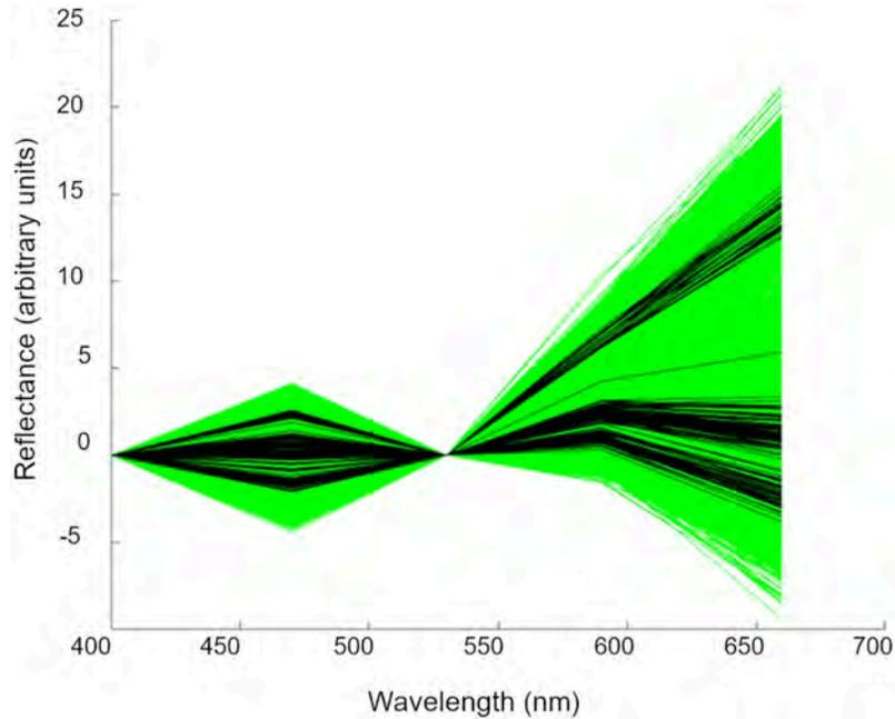
**Fig 2. Transformed spectral range.** Transformed image spectra of single seeds (green lines, n = 11309) and whole samples (black lines, n = 145). The single seed values are more extreme than the whole sample values.
