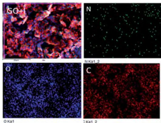
Fig. 2 Leucine functionalized graphene oxide elemental mapping.
