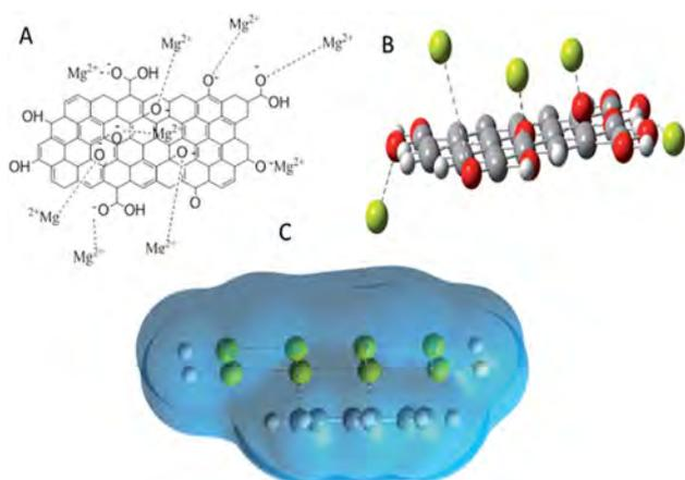
**Fig. 10** Proposed mechanism: (A) suggested physisorption of negative charged functionalized GO materials on Mg alloy surface, (B) depiction of Mg<sup>2+</sup> state-alloy surface electrostatic interaction, (C) total electrostatic interaction of functionalized graphene oxide materials on Mg alloy.
