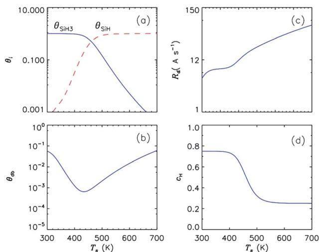
Fig. 2 Surface coverage of SiH and SiH<sub>3</sub> sites (a), surface coverage of dangling bonds (b), growth rate (c), and hydrogen content (d) as functions of substrate temperature. Other parameters are the same as in Table 1. The deposition rate increases quite slowly at temperature below 450 K, but then increases quicker as temperature rises above 450 K. The fraction of dangling bond sites also shows non-monotonic behaviour.
