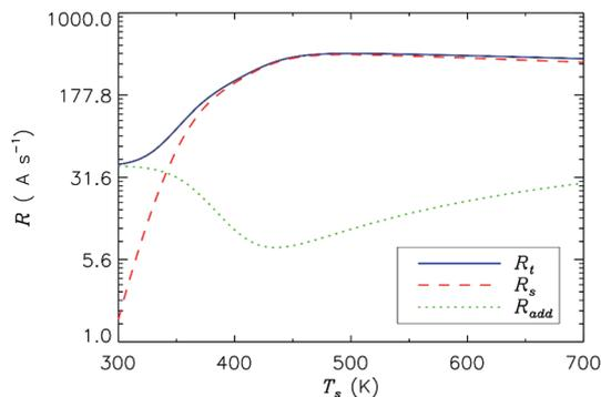
Fig. 3 Relative contributions of different pathways towards film growth under a typical deposition rate conditions. Other parameters are the same as in Table 1.  $R_s$ , chemisorption of physisorbed silyl radical to a dangling bond site;  $R_{add}$ , direct chemisorption into dangling bonds.
