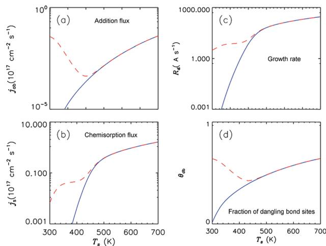
Fig. 4 Dependence of addition flux ( $J_{add}$ ), chemisorption flux of physisorbed radicals ( $J_s$ ), growth rate ( $R_d$ ), and fraction of dangling bond site ( $\theta_{db}$ ) on substrate temperature. The solid curves correspond to the case of the absence of ion sputtering, the dashed curves correspond to the cases in which the ion sputtering effect is taken into account. Other parameters are the same as in Table 1.
