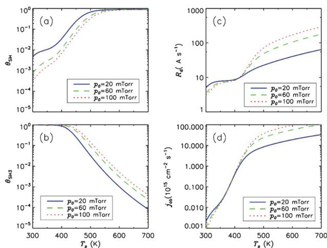
Fig. 6 Surface coverages of SiH<sub>3</sub>, H, and DB, and the film growth rate as functions of substrate temperature for three different pressures. Other parameters are the same as Table 1.
