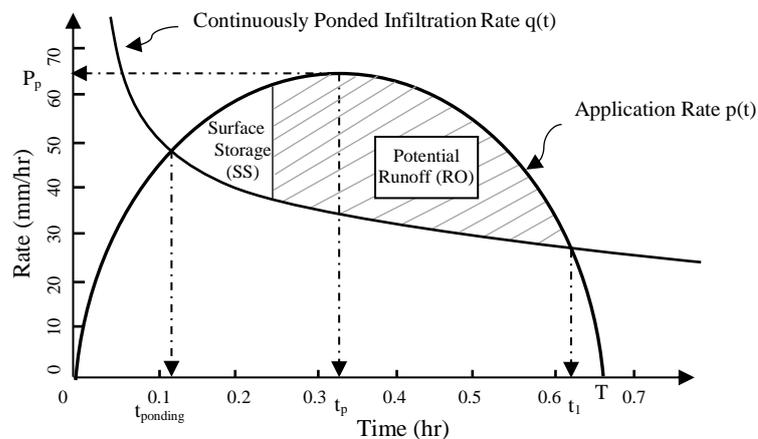
**Figure 1.** Application rate resulted from the overlap of individual sprinklers, adapted from [35].
