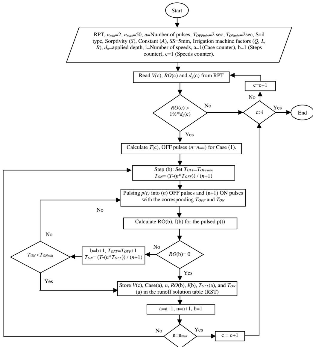
**Figure 4.** Flowchart for determining the runoff solution table (RST).
