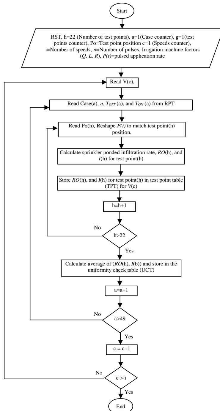
**Figure 5.** Flowchart for determining the uniformity check table (UCT).
