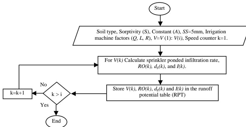
**Figure 2.** Flowchart for determining the runoff potential table (RPT).
