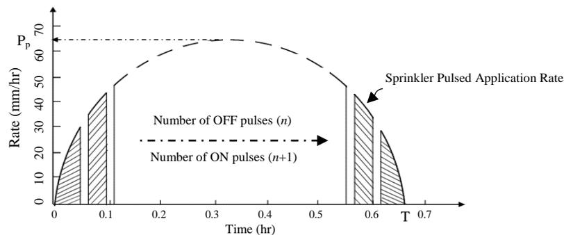
**Figure 3.** The suggested pulsation arrangement and its effect on the
