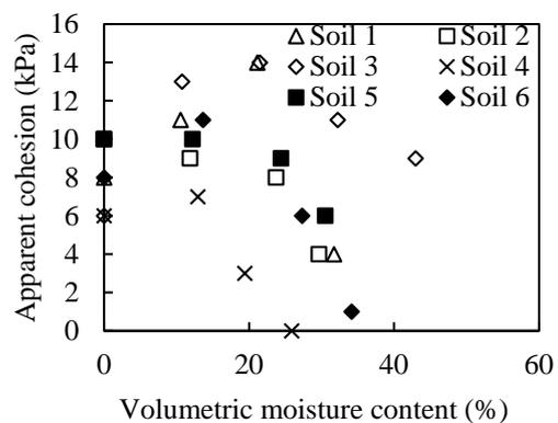
Fig. 2 Test results from shear box tests plotted as the apparent cohesion vs. volumetric moisture content.
