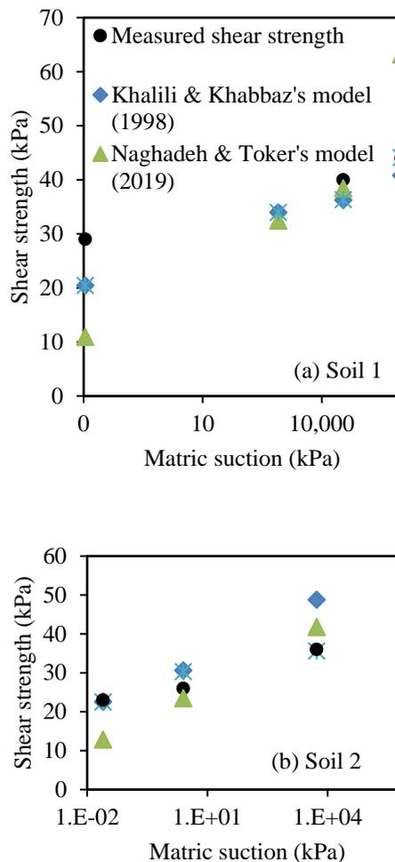
Fig. 6a and b Comparison of predicted shear strength with measured shear strength of Soils 1 and 2
