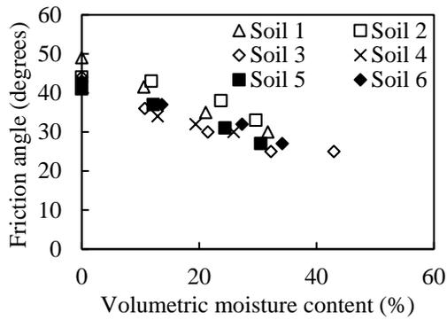
Fig. 3 Test results from shear box tests plotted as the friction angle vs. volumetric moisture content.
