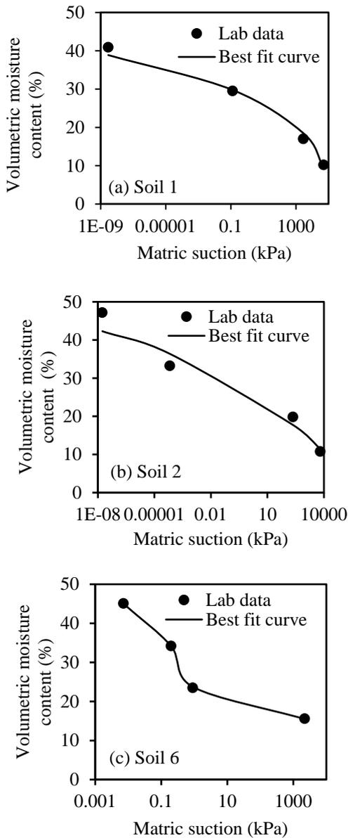
Fig. 5 Comparisons of the best fit SWCC models with the measured lab data.
