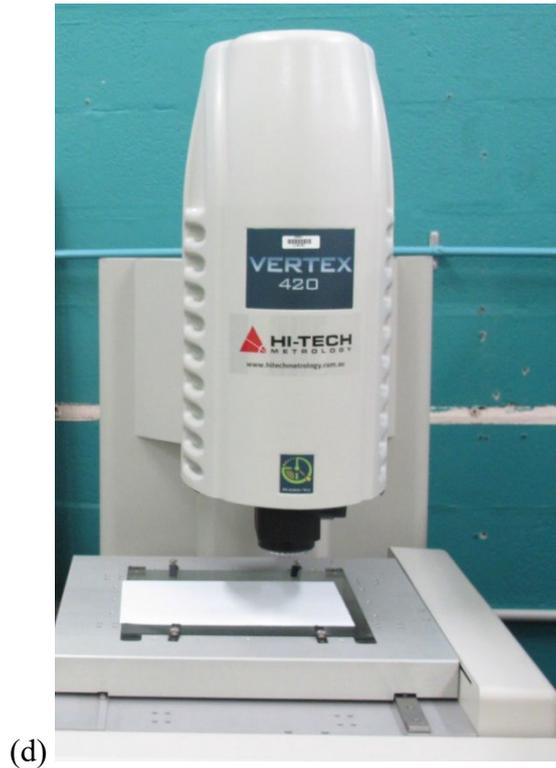
**Fig. 2. (a) Sample photo of the garnet particles under microscope; (b) Nozzle movement procedures in the AWJ drilling experiments; (c) a resultant blind hole; (d) Vertex 420 for hole diameter measurement**
