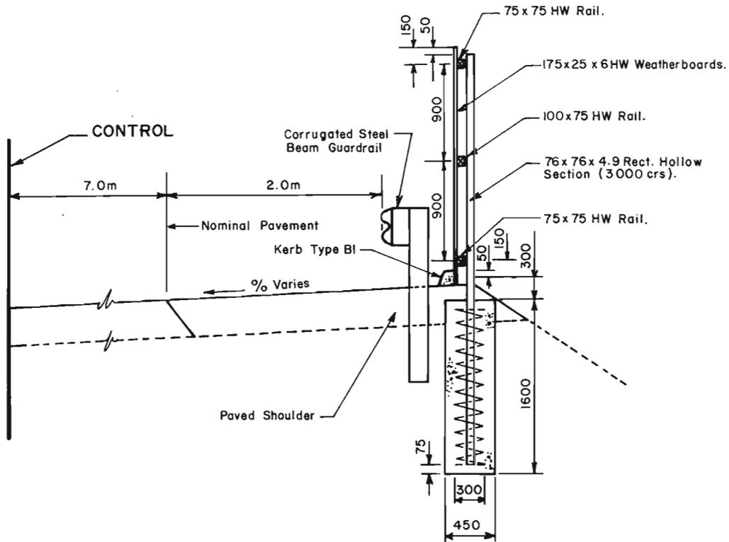
Fig. 3 - Typical Noise Fence Details
