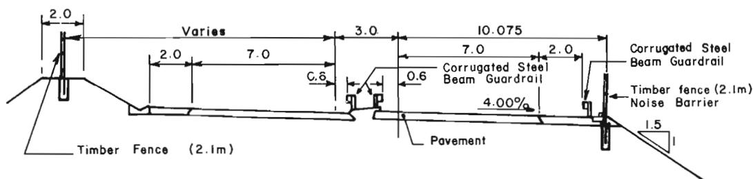
Fig. 2 - Typical Road Cross Section
