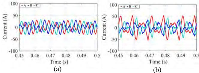
Fig. 12. Grid side harmonic currents (a) balanced harmonics (b) unbalanced harmonics.
