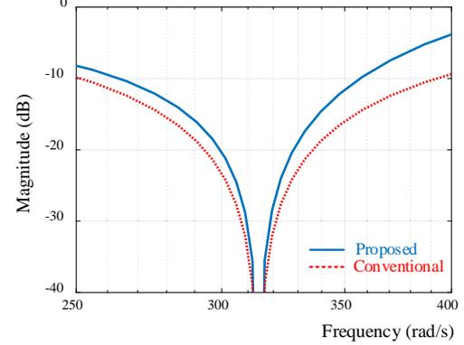
Fig. 4. The frequency response of the proposed method and the SOGI method: a) in generating  $u_\alpha(t)$  and  $\hat{u}_\alpha(t)$ , b) in generating  $u_\beta(t)$  and  $\hat{u}_\beta(t)$ .
