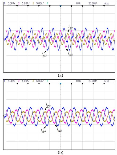
Fig. 19. Three-phase grid current under unbalanced loads condition (a) before compensation (b) after compensation. include different THDs of 21.4% and 36.2% respectively. The grid currents also follow the same THD to meet the load demands.
