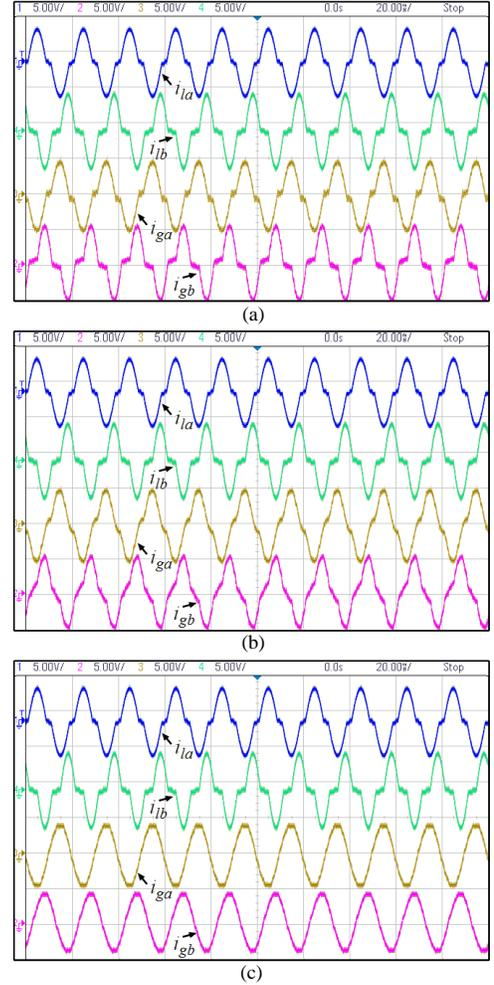
Fig. 18. Double-phase grid current with different degree of distortion (a) before compensation (b) compensation with conventional method (c) compensation with the proposed method.
