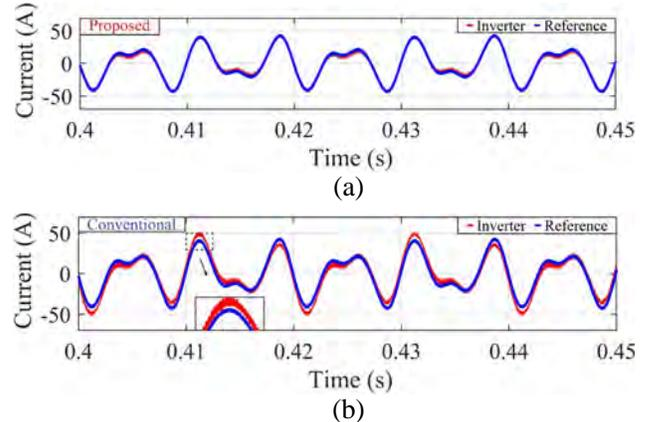
Fig. 10. Harmonics tracking performance (a) proposed three-arm inverter with split-capacitor arm (b) conventional three-arm inverter.
