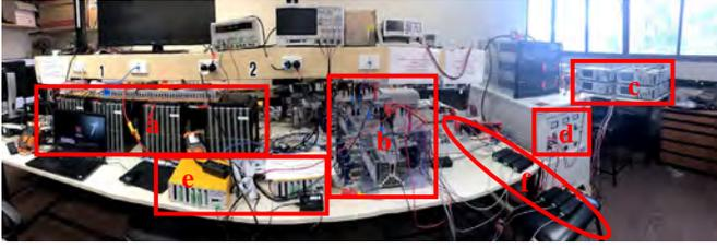
Fig. 16. Grid-connected microgrid system hardware configuration (a) batteries (b) Smart converter (c) Single-phase programmable loads (d) Transformer (e) DSP controller (f) Sensors and filter.
