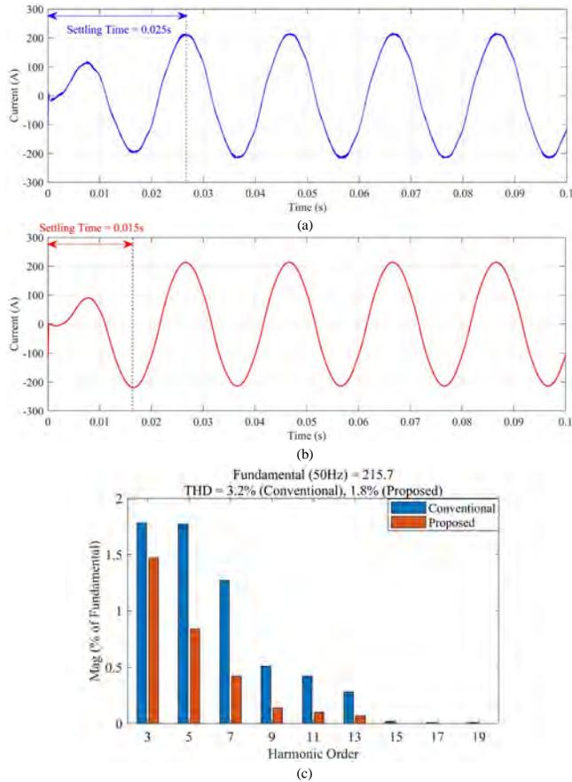
Fig. 8. a) Grid-side current while the conventional notch-filter based methods are used, b) Grid-side current while the proposed method is used, c) FFT analysis comparison between by the conventional NF and proposed NF.
