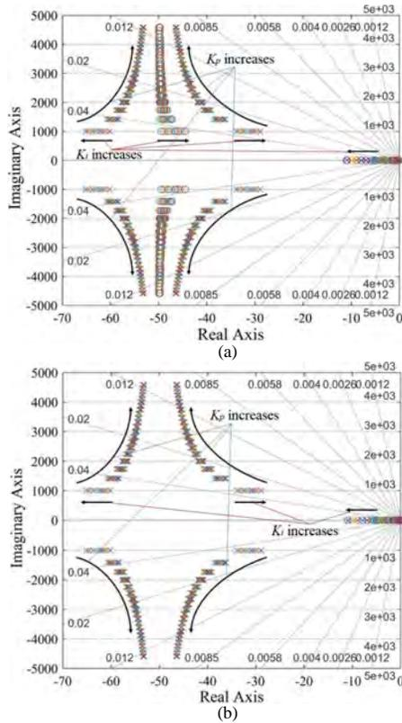
Fig. 6. Root locus for the  $i_{la}$  transfer functions a) corresponding to  $i_{od}$ , b) corresponding to  $i_{oq}$ .
