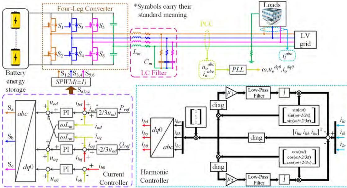
Fig. 1. Three-phase four-wire grid-connected microgrid system with the proposed control strategy.
