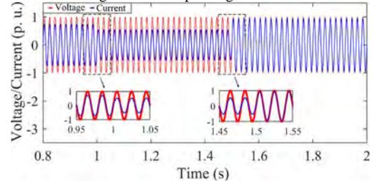
Fig. 15. Single-phase grid current variation due to the active power generation change of the microgrid.
