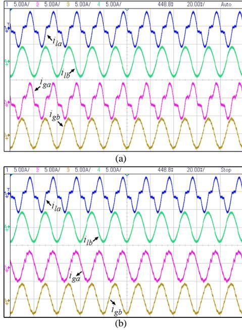
Fig. 17. Single-phase grid current (a) before compensation (b) after compensation.
