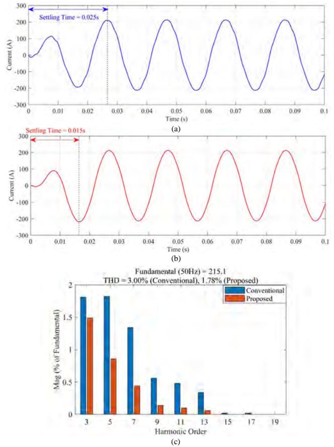
Fig. 7. a) Fundamental component generated by the conventional notch-filter based methods, b) Fundamental component generated by the proposed harmonics reduction method, c) FFT analysis comparison between by the conventional NF and proposed NF.
