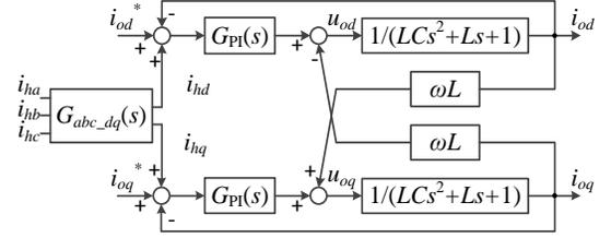
Fig. 5. Block diagram of the controller and plant in  $dq$  frame.
