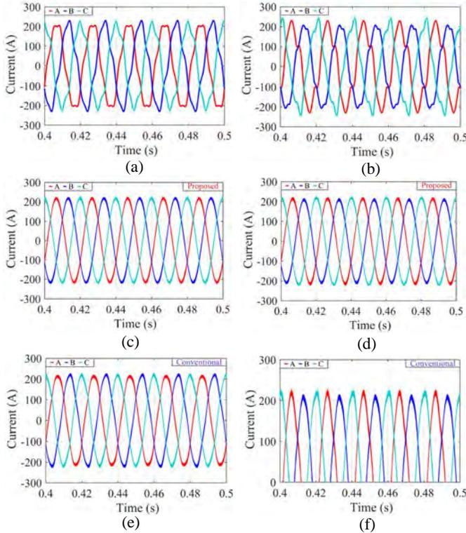
Fig. 11. Three-phase grid currents (a) balanced harmonics without compensation (b) unbalanced harmonics without compensation (c) balanced harmonics with proposed compensation (d) unbalanced harmonics with proposed compensation (e) balanced harmonics with conventional compensation (f) unbalanced harmonics with conventional compensation.
