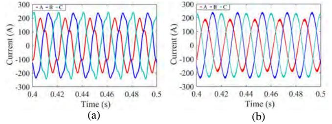
Fig. 9 Three-phase grid currents a) without compensation b) with compensation.
