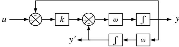
Fig. 2. The control algorithm of SOGI method.
