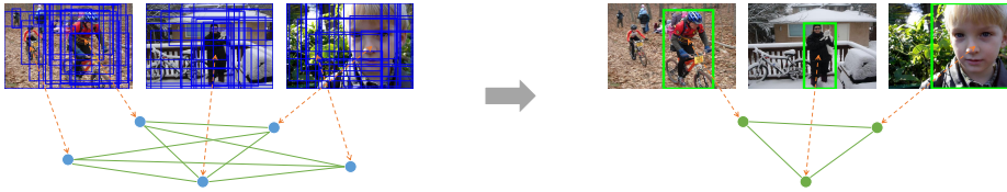
Fig. 1. Given a set of object candidates generated from an image collection (left), our goal is to find common objects by searching for the maximum weight clique in the associated graph. Each node in the clique (right) corresponds to a discovered common object.
