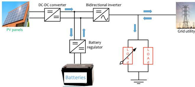
Fig. 1. A typical residential solar power system.
