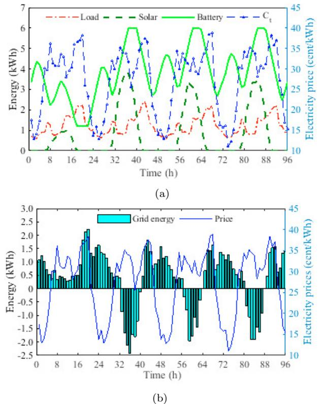
Fig. 6. Existing cost function: (a) charging/discharging cycles of the battery energy and (b) energy exchange with the grid.
