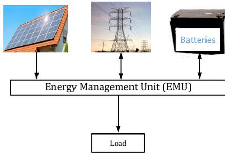
Fig. 2. Energy management unit for a residential PV system.
