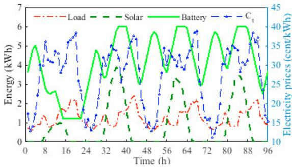
Fig. 7. Proposed cost function: optimal charging/discharging cycles of the battery energy.
