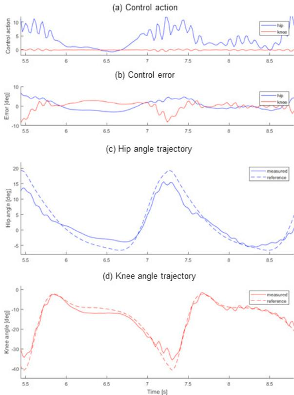
Fig. 4. Simulation results for 2 steps during permanent regime for the HNP control at  $0.3\text{ m/s}$  (gait period was  $1.76\text{ s}$ ). (a) Control signal for torque (hip, blue) and FES (knee, red) controllers. (b) Control errors. (c) Hip angle measurements and trajectory reference. (d) Knee angle measurements and trajectory reference.
