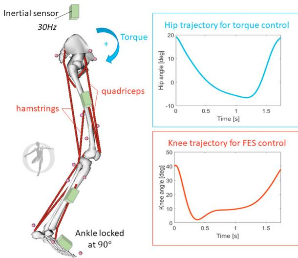
Fig. 1. The complete model for knee flexion and extension in OpenSim, representing the muscles as red lines. We locked the ankle joint at 90 degrees. The model also illustrates the hip and knee trajectory for the controllers. We represented the inertial sensors as blue cubes (on the trunk, upper leg, lower leg, and foot).
