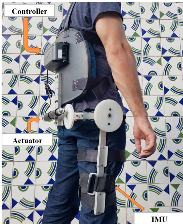
Fig. 2. The Hip Exosuit used by the volunteer. The ANT-38 actuator provides torque on the hip, while the Yost Labs IMU measures the hip angle position.
