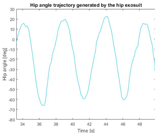
Fig. 5. Experimental results for the active orthosis (gait period was  $5.35\text{ s}$ ).
