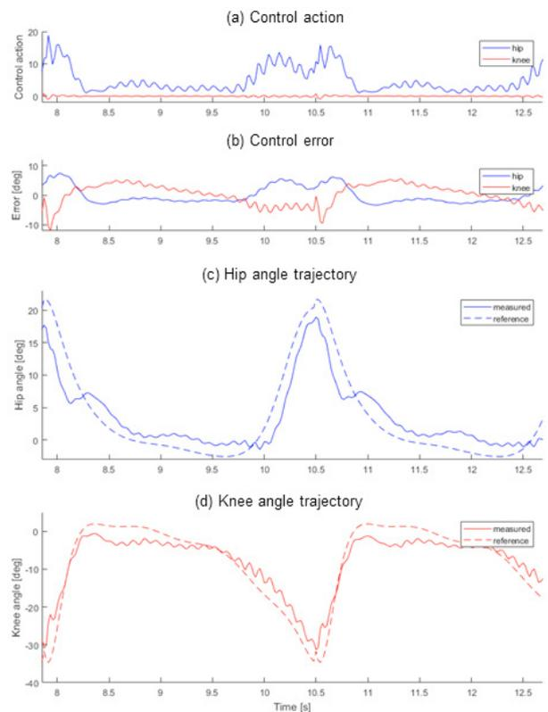
Fig. 3. Simulation results for 2 steps during permanent regime for the HNP control at  $0.1\text{ m/s}$  (gait period was  $2.54\text{ s}$ ). (a) Control signal for torque (hip, blue) and FES (knee, red) controllers. (b) Control errors. (c) Hip angle measurements and trajectory reference. (d) Knee angle measurements and trajectory reference.
