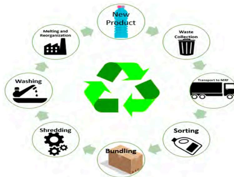
**Figure 1.** The typical stages involved in plastic recycling.
