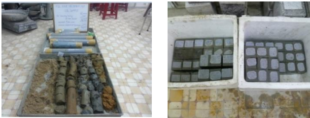
A. Prepared soil for casting B. Curing sample
