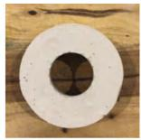
b- Top view of set plaster mould with circular hole
