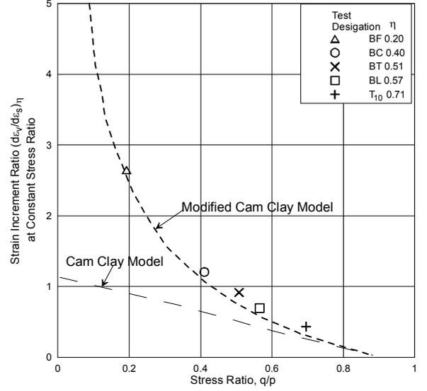
Fig. 4 Observed and predicted dilatancy ratio (Balasubramaniam, 1969)
