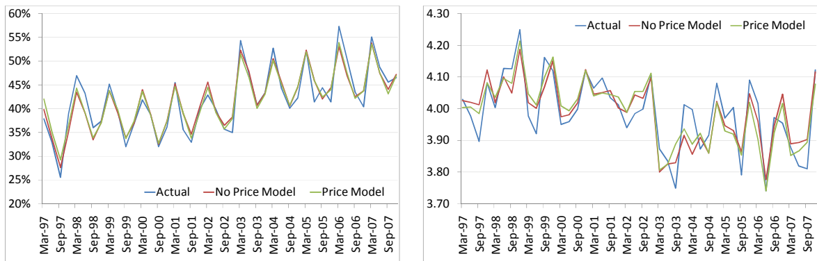
Figure 5 Actual and fitted values of quarterly weighted average propensity to use car (left) and log of car kilometres per night among tourists who used cars (right).
