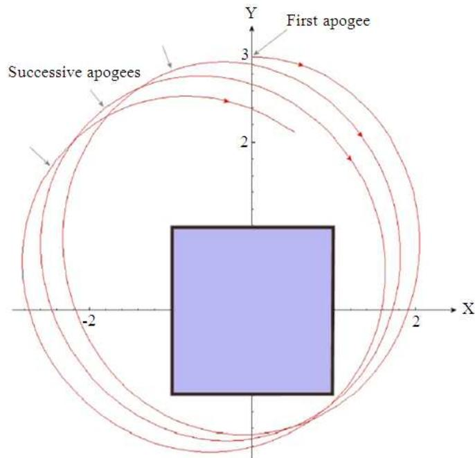
**Fig. 4.** A satellite orbiting around the equator of a static cube with a side length equal to the diameter of the Earth. Beginning with an satellite orbital radius of three Earth radii and a velocity of  $3.63 \text{ km s}^{-1}$ , we find a period of approximately 4.8 h, but with an orbit that precesses fairly rapidly, as shown by the counterclockwise movement of successive apogees
