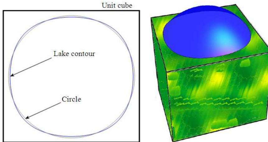
**Fig. 1.** A lake formed on the surface of a cube. As expected, the edge of the lake is ‘pulled up’ towards the corners, due to the extra mass present there, but forming a nearly spherical surface
