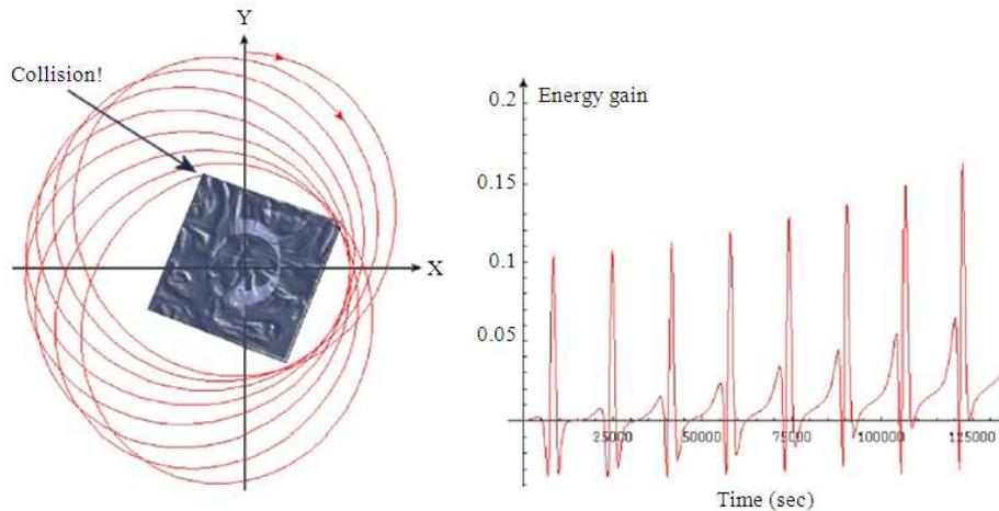
**Fig. 6.** Orbits around a cube rotating with a 10 h. day, with a 4.8 h. satellite orbit, close to a 2:1 resonance. With this configuration we find that the satellite rapidly acquires energy, colliding with the cube near the end of the eighth orbit as shown. From the graph of energy gain, we can see that by the 8<sup>th</sup> orbit the satellite has a nearly 17% energy gain at perigee
