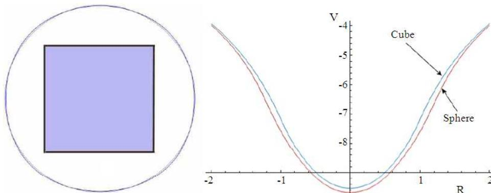
**Fig. 3.** The equipotential around the equator of the cube. Notice how the field is slightly stronger over the corners, indicated by the equipotential being shifted outwards compared to a perfect circle. When comparing the gravitational potential of a cube to a sphere of the same mass, because the sphere is a more compact object we find a deeper potential well, though the two potentials converge at larger distances as expected
