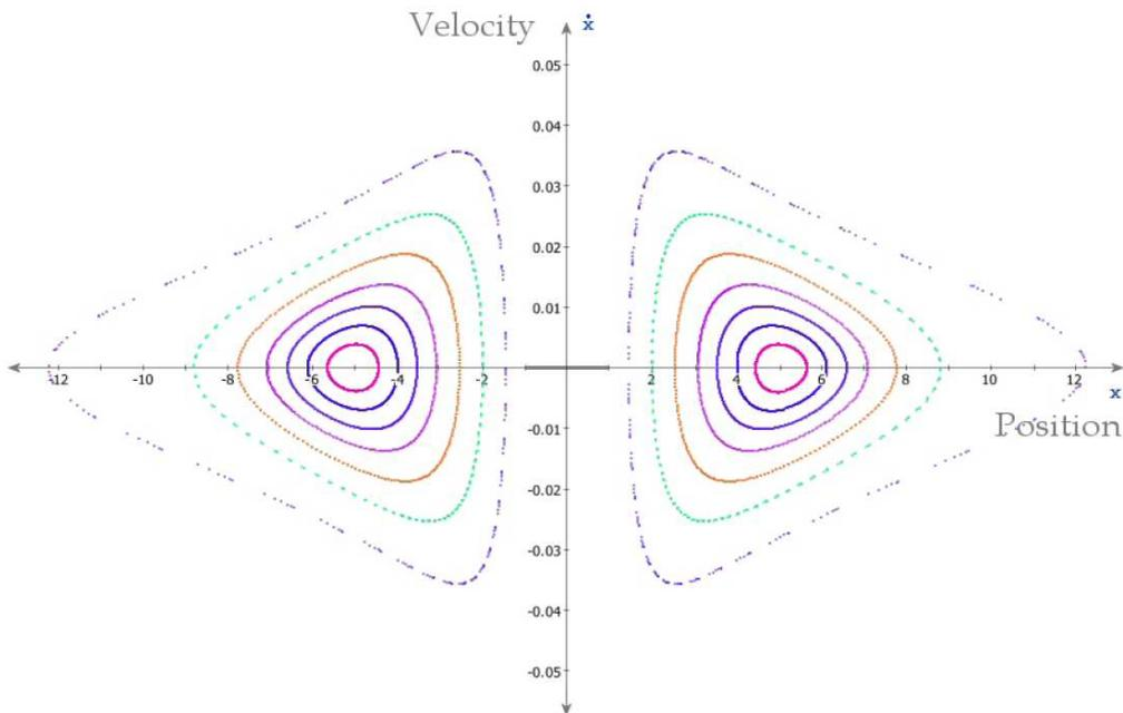
**Fig. 5.** The Poincaré section, plotting the  $x$  coordinate (when  $y = 0$ ) against its velocity in the  $x$  direction, for satellites around the unit cube showing a closed orbit for this particular satellite energy at approximately five units
