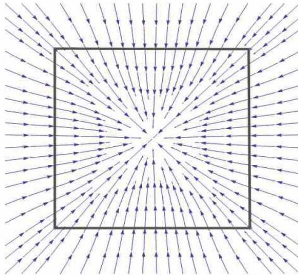
**Fig. 2.** The field through a cube sliced in half through the faces. We can observe the slight distortion of the field lines between the edges and the center of each face
