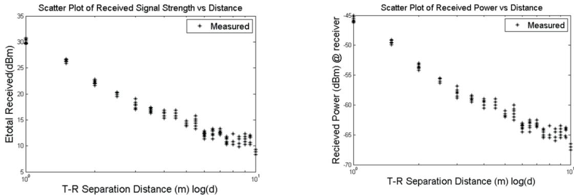
Fig. 2. Signal strength data recorded for all paths. a) Received field strength vs. Log-distance; b) Received power vs. Log-distance
