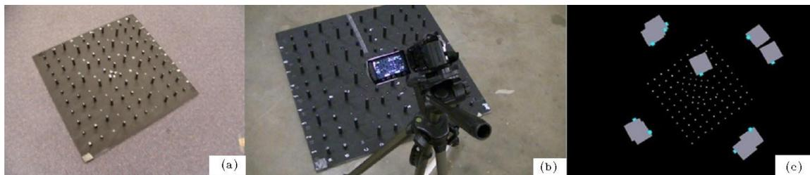
Figure 2. (a): calibration test-field; (b): video camera calibration setup; (c): Image acquisition geometry. Note the camera shutter button position.
