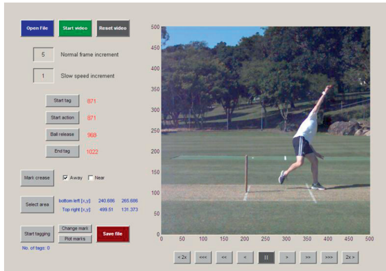
Fig. 3. Video digitising interface snapshot of the elbow’s/wrist’s marker-based system.
