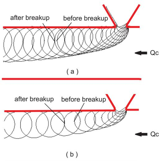
**Figure 4.** Measured formation process of ferrofluid in the absence of an external magnetic field ( $Q_d = 10 \mu\text{l/hr}$ , delay time between each frame 0.08 sec): (a)  $Q_c = 50 \mu\text{l/hr}$ ; (b)  $Q_c = 100 \mu\text{l/hr}$ .
