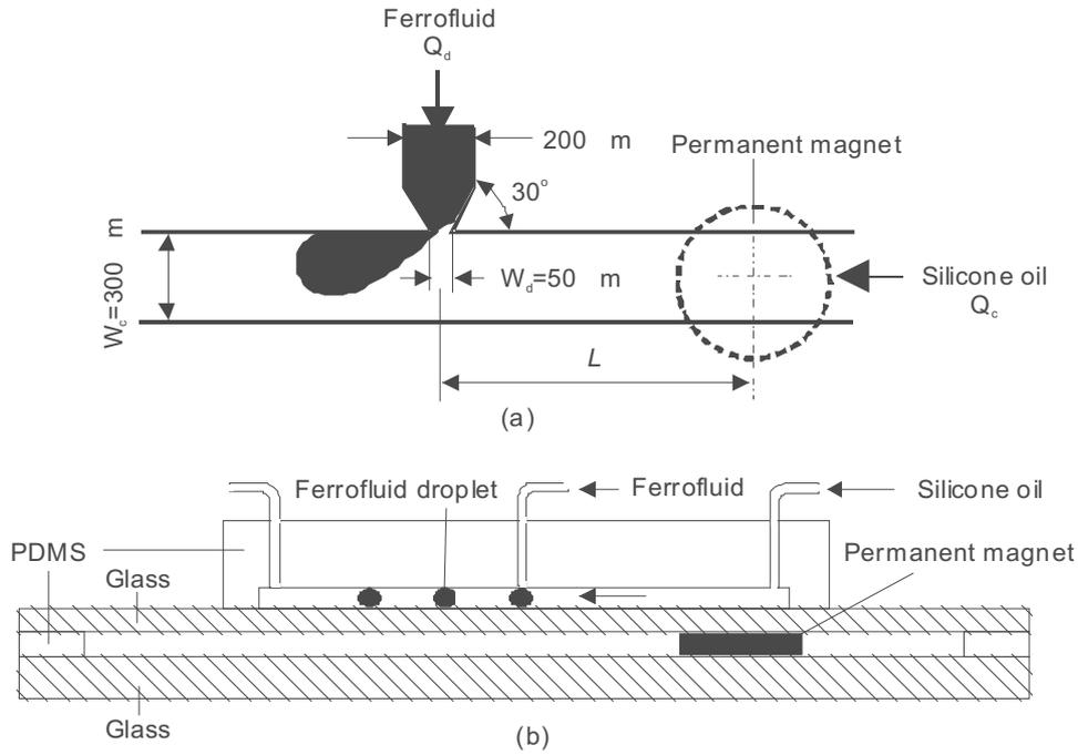
**Figure 2.** Schematics of the experimental setup for the formation of ferrofluid droplets at a microfluidic T-junction (not to scale): (a) The microfluidic network; (b) The setup with the permanent magnet. The PDMS layer separating the glass and magnet in Fig. 2(b) acts as a support for the microfluidic chip. It has the same thickness of approximately 2 mm as the magnet.
