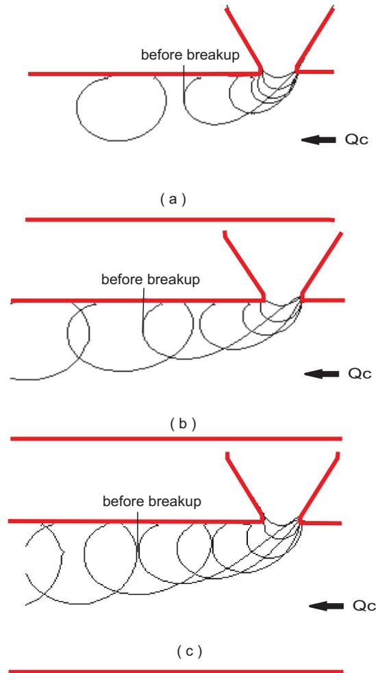
**Figure 9.** Measured formation process of ferrofluid at  $Q_d = 10 \mu\text{l/hr}$  and  $Q_c = 100 \mu\text{l/hr}$ . (delay time between each frame 0.08 sec) The magnet is placed at different downstream positions: (a) at a distance of 2.3 mm ( $B = 27.2 \text{ mT}$ ); (b) at a distance of 2.8 mm ( $B = 22.0 \text{ mT}$ ); (c) at a distance of 3.8 mm ( $B = 13.4 \text{ mT}$ ).
