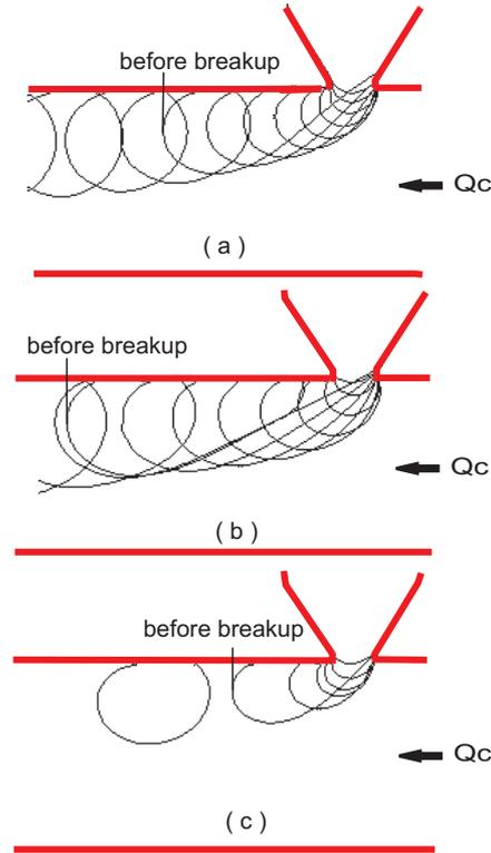
**Figure 5.** Measured formation process of ferrofluid droplets at  $Q_d = 10 \mu\text{l/hr}$  and  $Q_c = 100 \mu\text{l/hr}$  (delay time between each frame 0.08 sec): (a) without permanent magnet; (b) permanent magnet upstream at a distance of 2.3 mm ( $B = 27.2 \text{ mT}$ ); (c) permanent magnet downstream at a distance of 2.3 mm ( $B = 27.2 \text{ mT}$ ).
