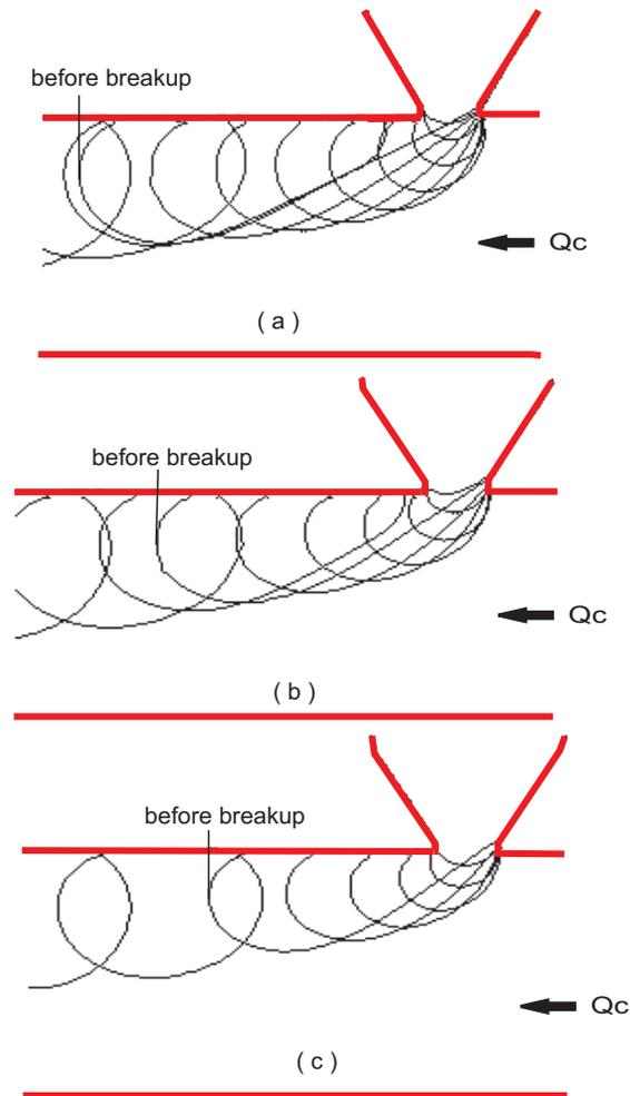
**Figure 8.** Measured formation process of ferrofluid at  $Q_d=10 \mu\text{l/hr}$  and  $Q_c = 100 \mu\text{l/hr}$ . (delay time between each frame 0.08 sec) The magnet is placed at different upstream positions: (a) at a distance of 2.3 mm ( $B = 27.2 \text{ mT}$ ); (b) at a distance of 2.8 mm ( $B = 22.0 \text{ mT}$ ); (c) at a distance of 3.8 mm ( $B = 13.4 \text{ mT}$ ).
