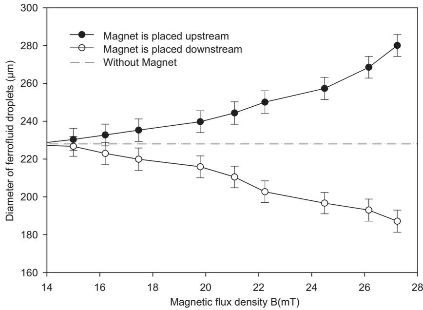
**Figure 7.** Diameter of ferrofluid droplet as function of magnetic flux density for both upstream and downstream cases. The dashed line represents the diameter of the formed droplets in the absence of the magnet. In all the three cases, the flow rate of the dispersed phase is fixed at  $Q_d = 10 \mu\text{l/hr}$  and the continuous phase is fixed at  $Q_c = 100 \mu\text{l/hr}$ .
