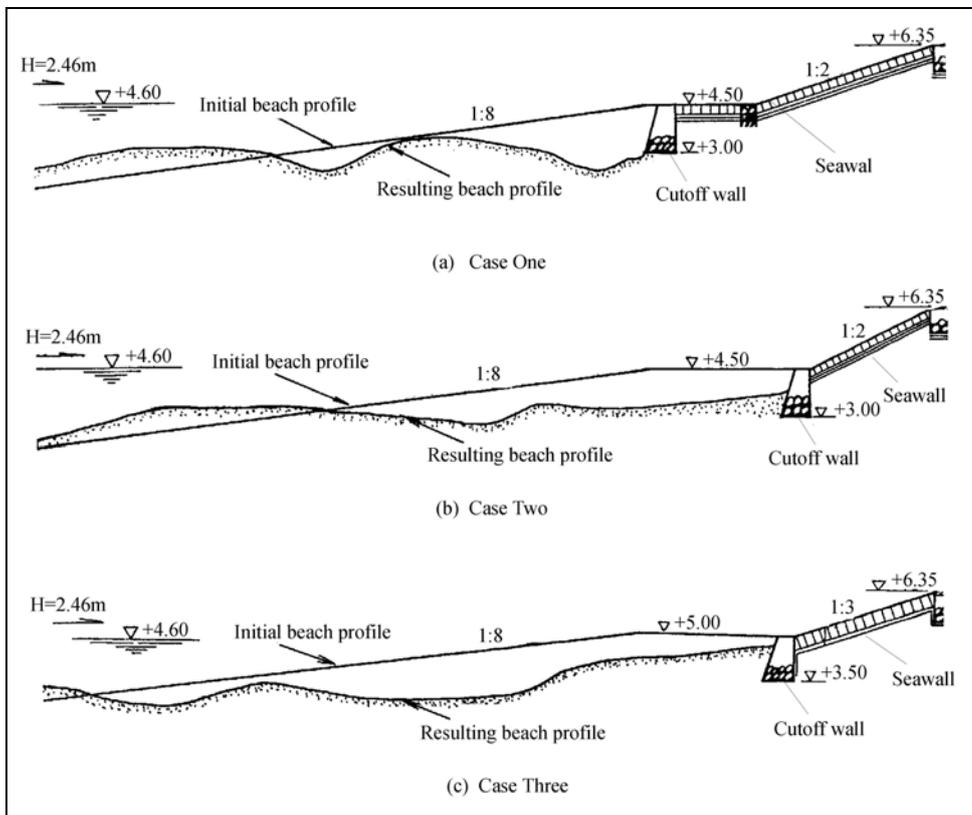
Figure 2. Resulting profile configurations with different kinds of seawalls under erosive wave conditions with a 50-year return period. An initial profile with a face slope of 1:8 was determined by the situation of artificial sandy beaches on the coast of Northern Jiangsu Province, China. Each test was run for a 24 hours prototype wave action.
