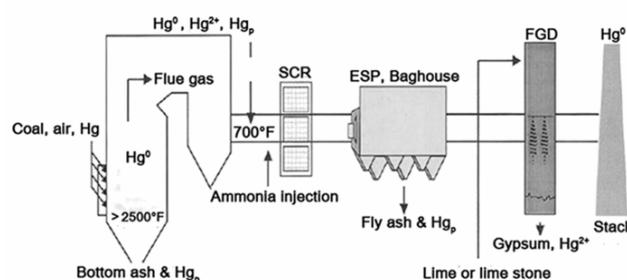
**FIGURE 1 - Hg distribution in coal combustion. Hg distributes in bottom ash, fly ash and gypsum in the process of coal firing. The speciation of Hg in combustion includes Hg<sup>0</sup>, Hg<sup>2+</sup>, Hg<sub>p</sub>.**
