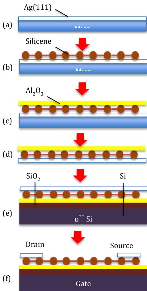
Figure 1. Fabrication steps of the silicene transistor
