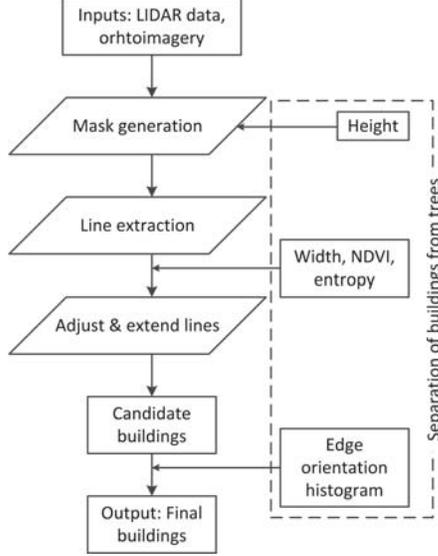
Fig. 1. Proposed building detection technique.
