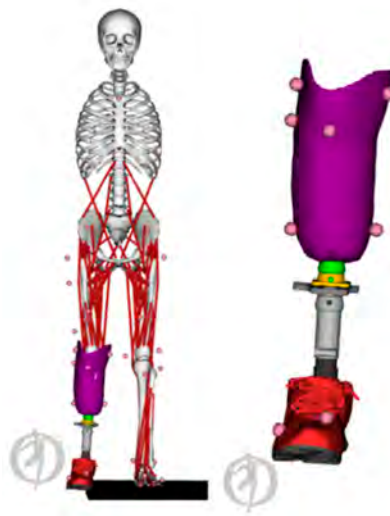
Figure 6. Example of a MSK model implemented in OpenSim which includes a model of a transtibial prosthetic device [102].
