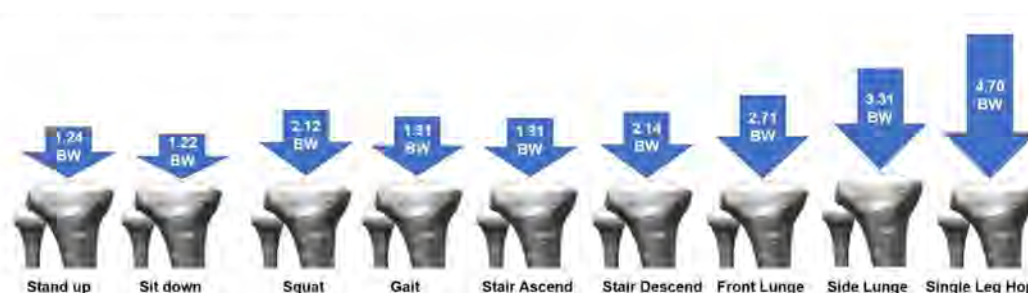
Figure 5. Average tibiofemoral joint contact forces for a range of different functional and rehabilitation tasks [63].
