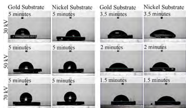
Fig. 10 Contact angle images for all samples produced.
