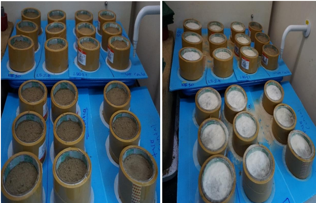
838 Figure 5: Treatment of sand column using locally isolated bacteria, consortia, 839 positive and negative controls. (a) setup of sand columns before treatment with 840 ureolytic bacteria and cementation solution (Left). (b) sand columns during 841 treatment with bacteria and cementation solution (right).
