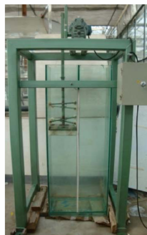
FIGURE 1 - Vertical oscillation-making device (units: cm).
