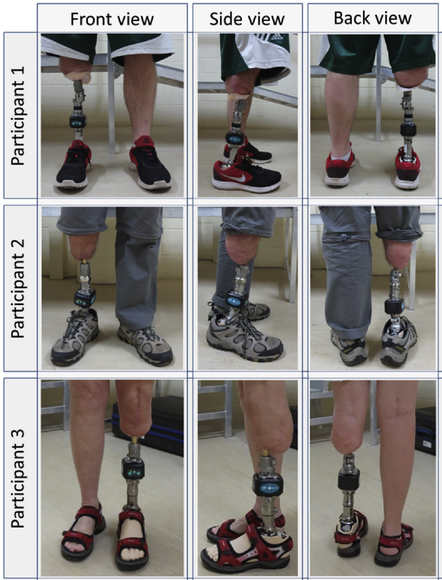
Fig. 1. Inter-participant variability of alignment and position of the tri-axial transducer (iPecLab, RTC, US) in relation to the ankle joint embedded in the instrumented transtibial bone-anchored prosthesis fitted with Free-Flow Foot (Ohio Willow Wood).
