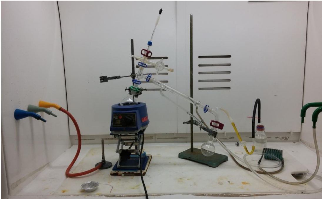
Figure 28: Experimental set-up showing the glass pyrolysis reactor, electric heating system, condensation train, gas sampling, oil collection and vacuum cooling system.
