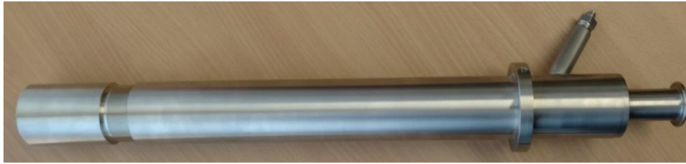
Figure 32: Steel reactor tube inlet
