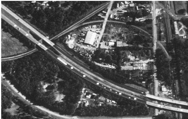
Fig. 8. Road tracking from upper left to lower right. White dots are the detected road axis points, white line segment shows the location of human input. The number of human inputs is reduced by searching multiple reference profile lists, as described in the text.
